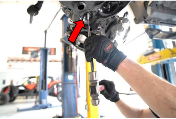
13. The lower shock mount bolts are pressed into the lower shock mount, so you will need to use a drift and a hammer to remove the lower shock mount bolts.
