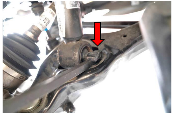
16. Pry under the right side of the bar pin and be careful not to pry the shock into the CV boot as this WILL rip the cv boot.
