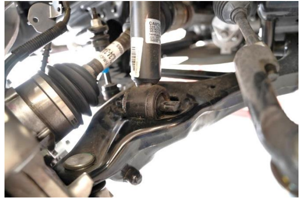
14. OE lower shock mount bolts removed from the lower shock mount.
