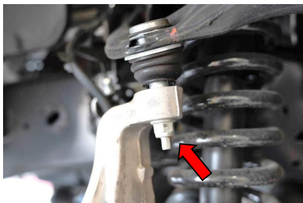
9. Loosen but DO NOT remove the nut for the upper top ball joint with an 18mm wrench.
