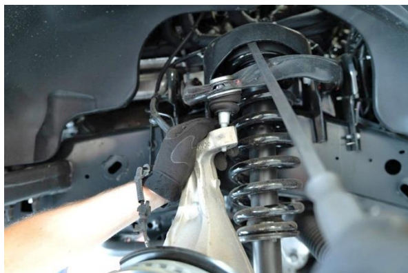
11. Slowly let the control arm upwards to release the ball joint from the knuckle.
