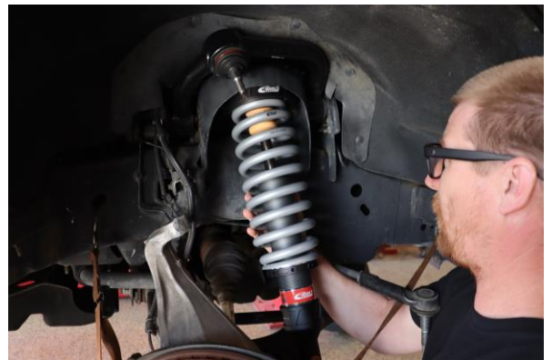
18. Install EIBACH PRO-TRUCK COILOVER 2.5.
