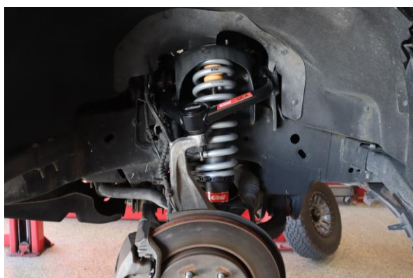
27. Install wheel and repeat instructions to other side. Vehicle will require alignment after installation of kit. shocks
