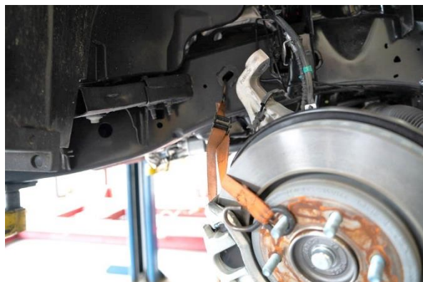
12. Use a tie strap to keep the knuckle from drooping down.
