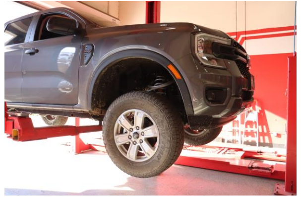
20. Install the wheel and tire using 19mm. Tighten to manufacturer specification.
