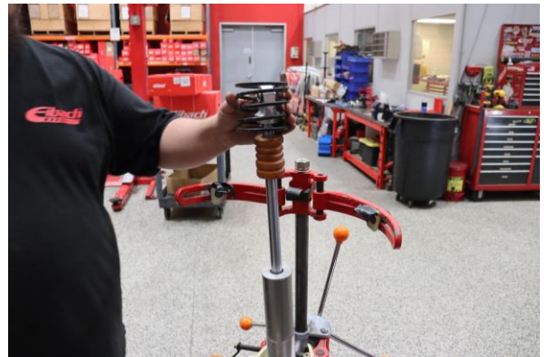
Step 14. Remove the second OE tender spring.
