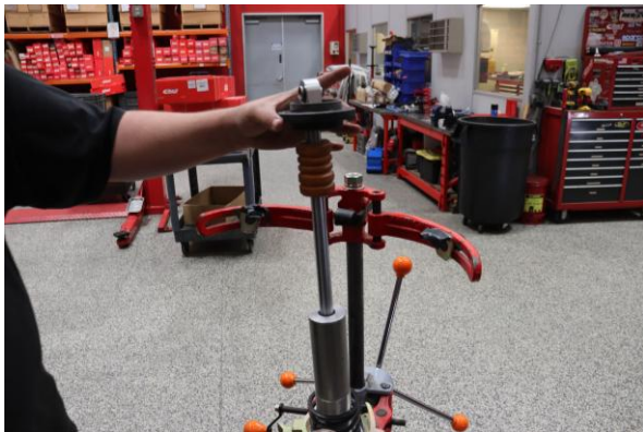
Step 13. Remove the second OE spring slider.
