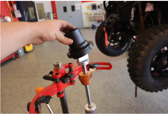
Step 9. Remove the OE spring slider.
