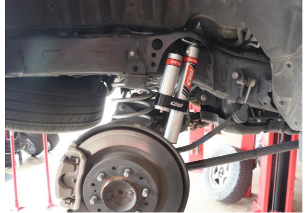
(RIGHT SIDE) shown above with reservoir facing axle/rear of vehicle. 82135.8004RR-R
