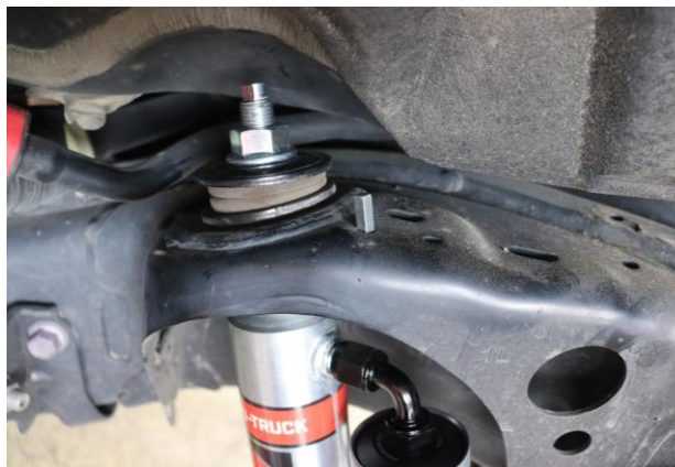
Insert metal tab into outermost slot as shown above.
