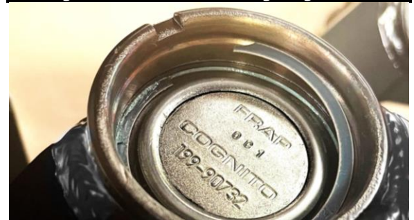
Figure 4: Internal Retaining Ring Install
