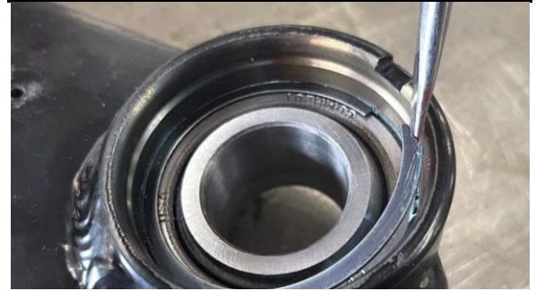
Figure 2: Internal Retaining Ring Removal
