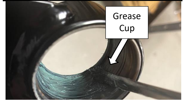
Figure 3: Deburr and Grease
