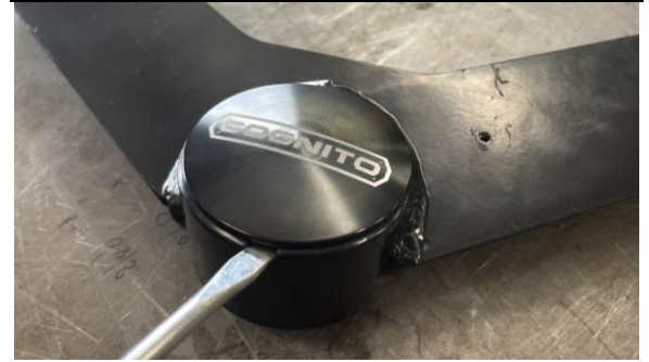
Figure 1: UCA Cap Removal
