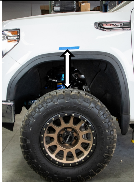
Figure 5: Measuring and Setting Ride Height
