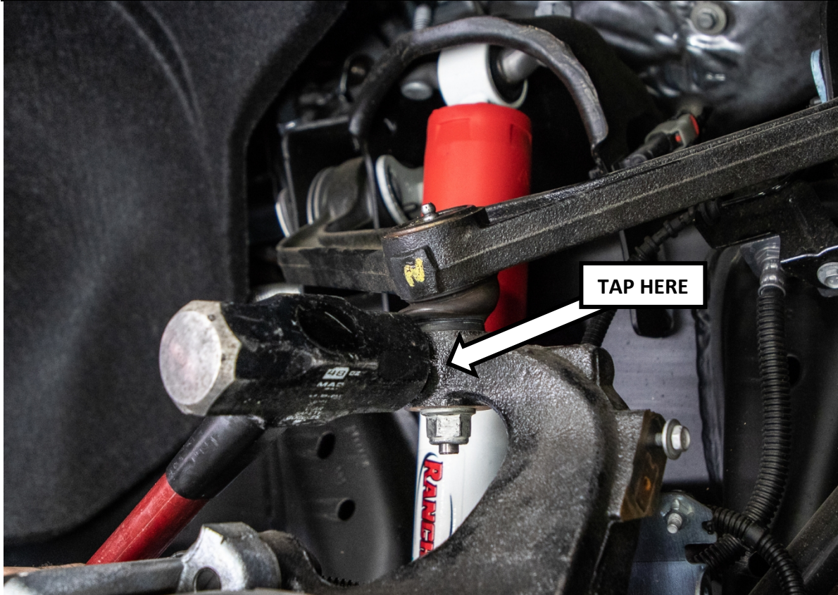
Figure 2: UCA and Spindle Disassembly
