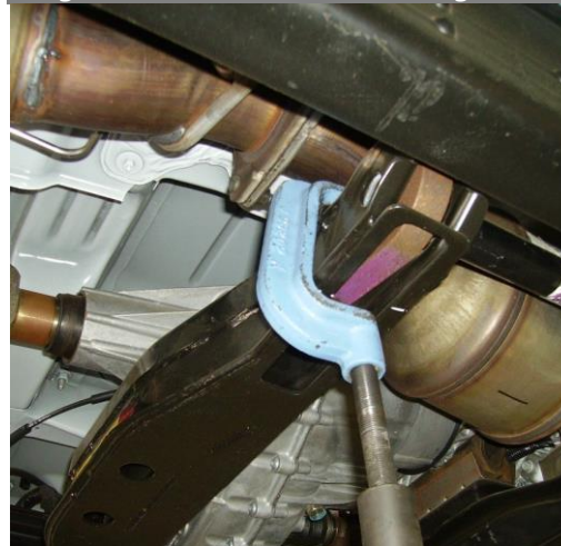
Figure 2: Load Torsion Bar Using Tool
