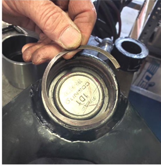
Figure 3: Internal Retaining Ring Removed
