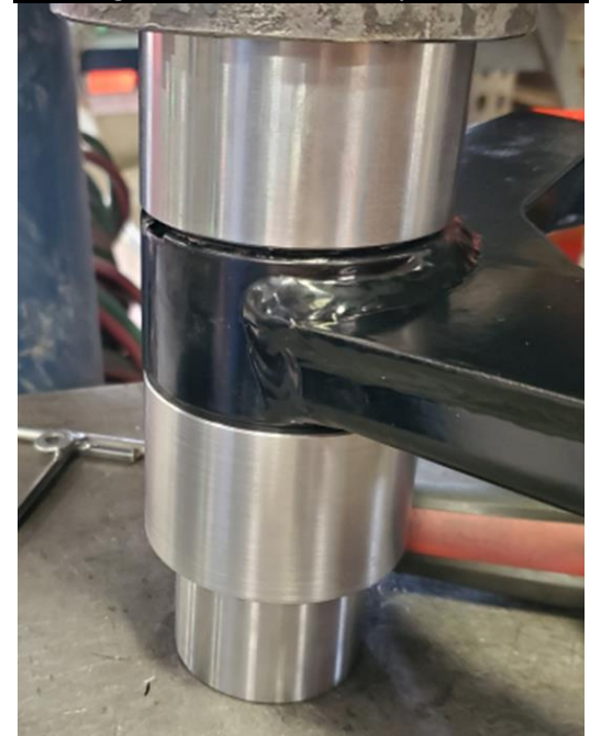
Figure 11: Ball Joint Fully Seated
