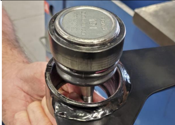
Figure 8: Place New Ball Joint into Arm
