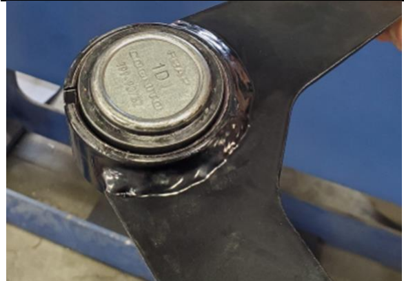
Figure 9: Ball Joint prior to Pressing
