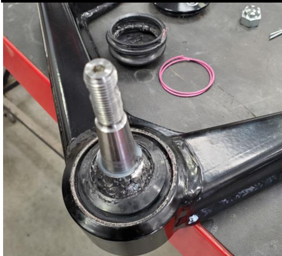
Figure 4: Dust Boot & Wire Retaining Ring Removed
