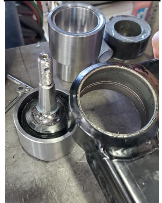
Figure 6: Ball Joint Pressed Out
