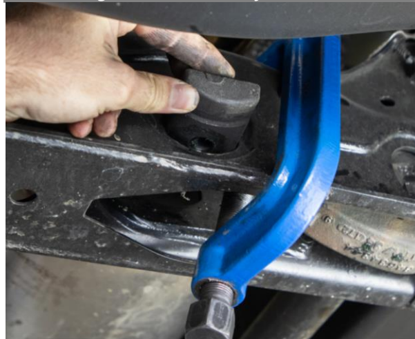
Figure 3: Remove Adjuster Nut
