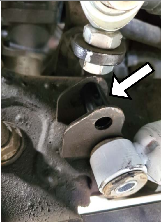
Figure 1: Crush Sleeve Installed
