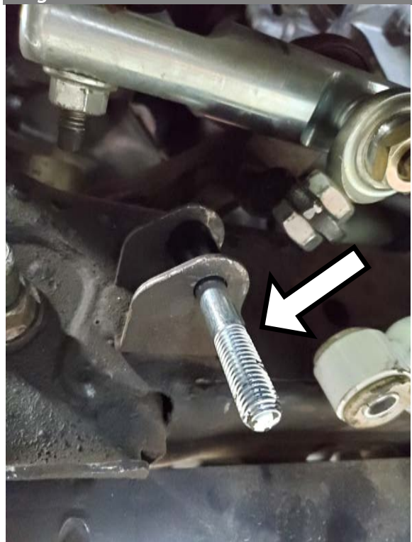
Figure 2: Bolt Installed on Frame Mount
