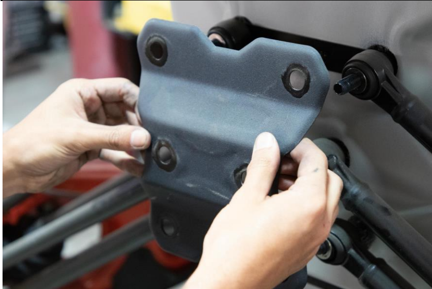
Figure 2: Remove radius rod plates.
