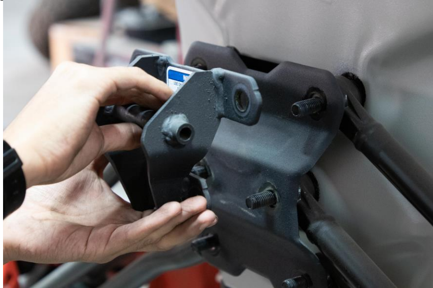
Figure 1: Remove radius rod plates.
