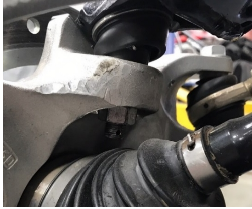
Figure 1: Remove nut and washer off bottom side of ball joint
