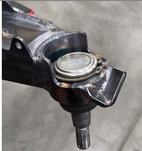
Figure 3: Ball joint pressed into Cognito arm.
