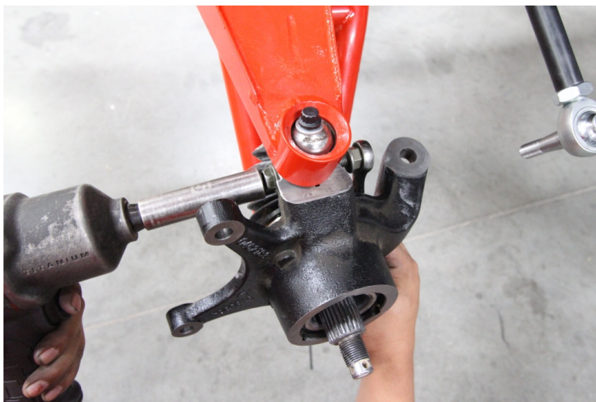
Figure 2: Tighten stud with pinch bolt.
