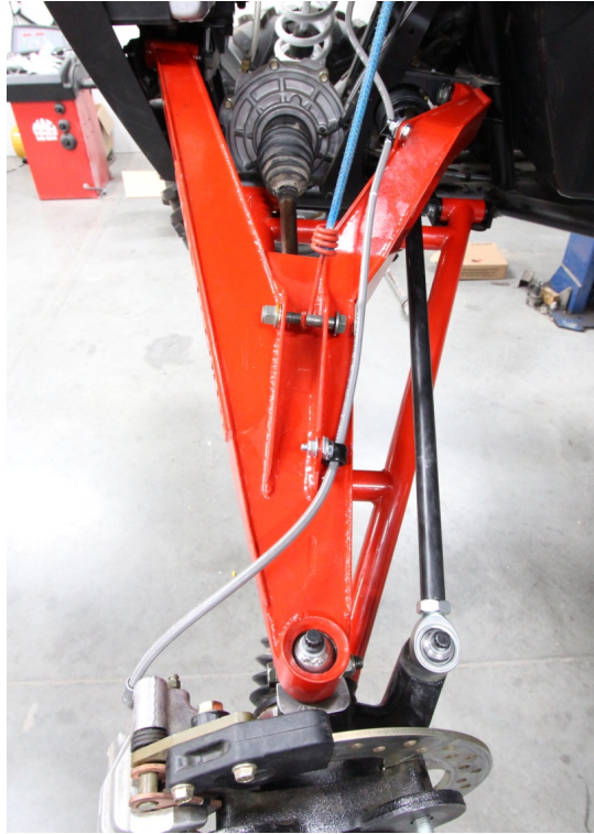
Figure 4: Fasten brake line with cushion clamps.
