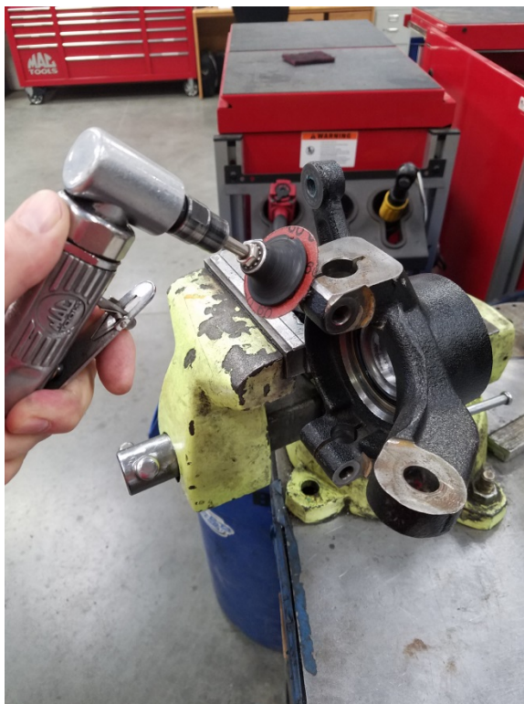
Figure 1.2: Sanding the edge.
