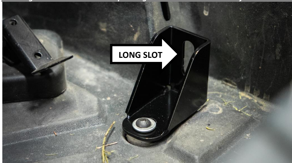
Figure 5: 8754 installed on passenger side. Note orientation of bracket.
