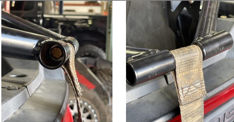
Figure 16: Connect swing frames together with supplied hardware.
