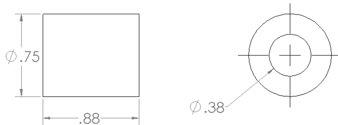
Figure 4: Aluminum spacer 5030 dimensions.
