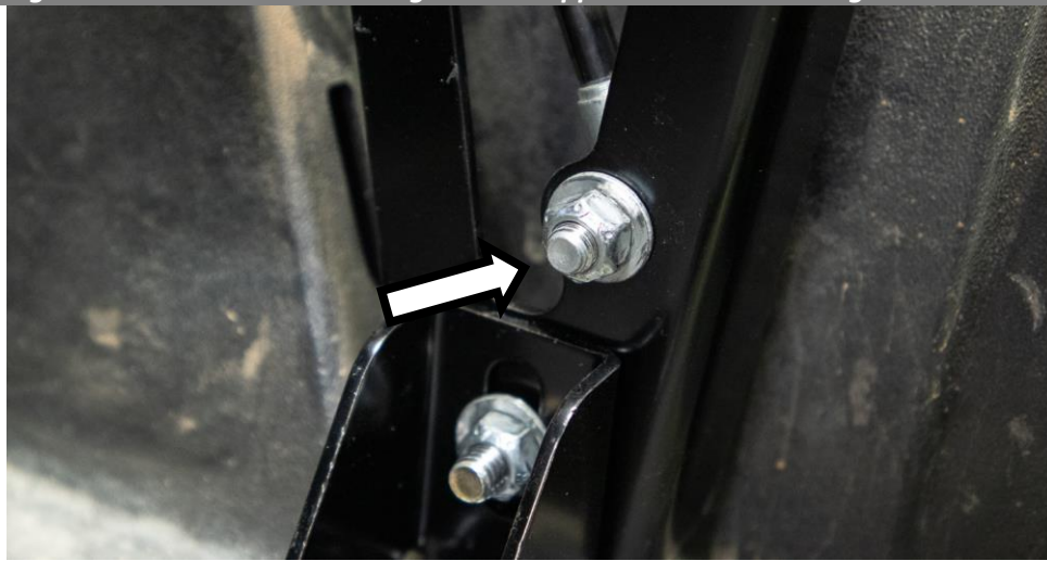
Figure 26: Insert rod end through lower support bracket. Passenger side shown.
