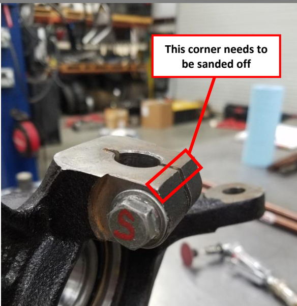
Figure 3: More detailed note of the trimming, which must be done to both areas shown in Figure 1
