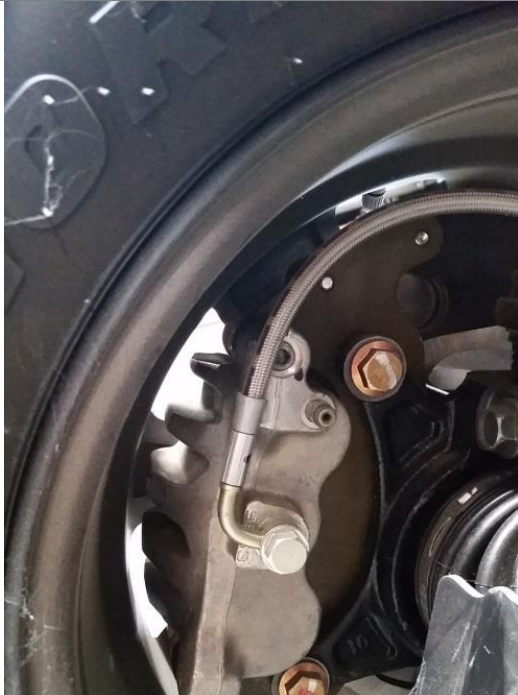
Figure 10: This is stock. The brake line fitting is far from the bleeder screw. This kicks the brake line up close to the wheel.
