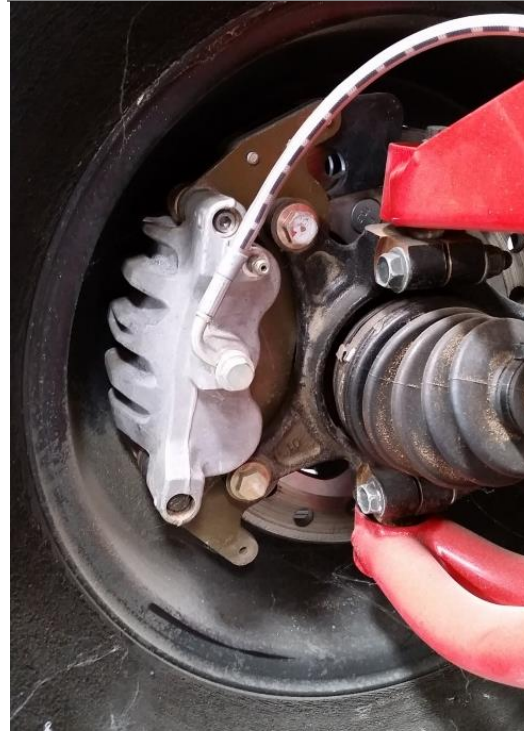
Figure 11: Brake line is closer to the bleeder but farther from the wheel.
