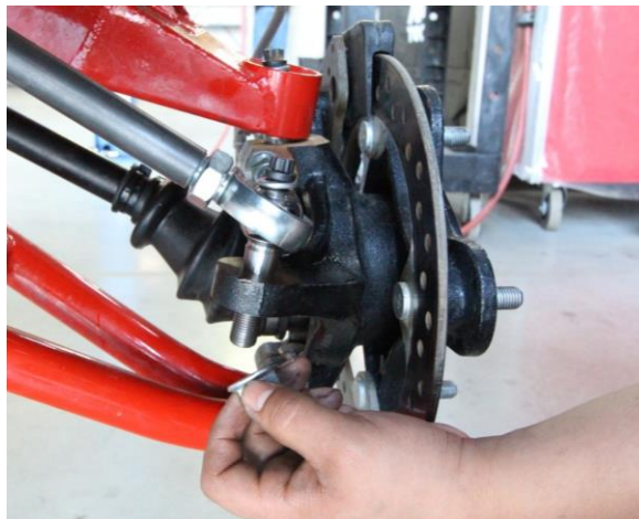
Figure 6: Shows the stud in the spindle, rod end on the stud, then spherical washer on the rod end held in place by lock washer and 12 point bolt
