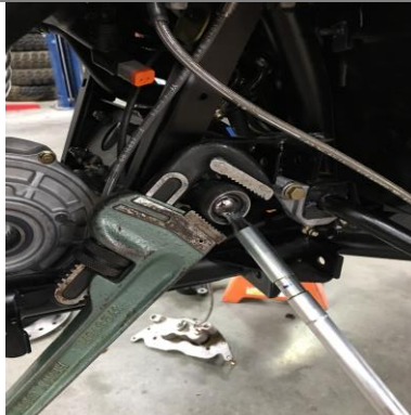
Figure 1: pull dust boot back, remove inner tie rod from rack bar
