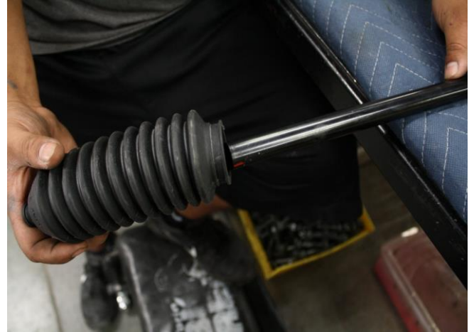
Figure 2B: Install boot
