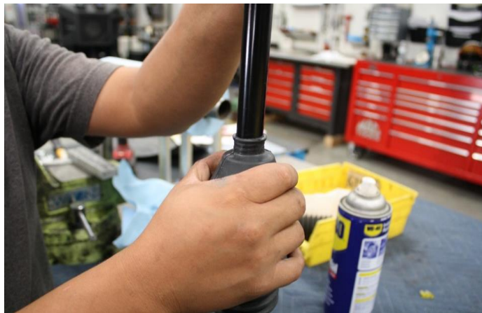
Figure 3C: Pull boot down
