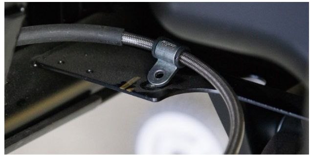
Figure 1B: Mounting Bolt Removed
