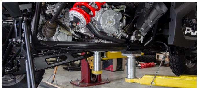
Figure 13B: Trailing Arm Removed
