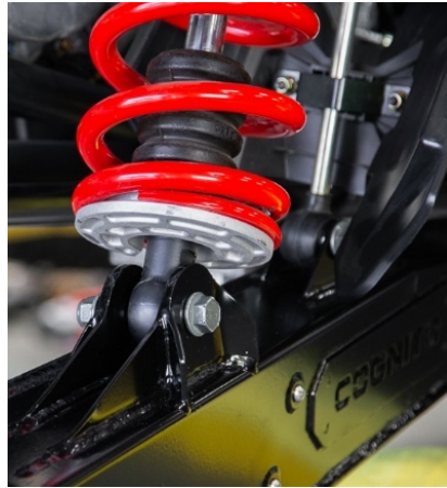
Figure 17B: Shock Installed
