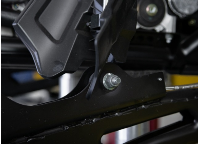
Figure 5A: Rear Sway Bar End Link Removal
