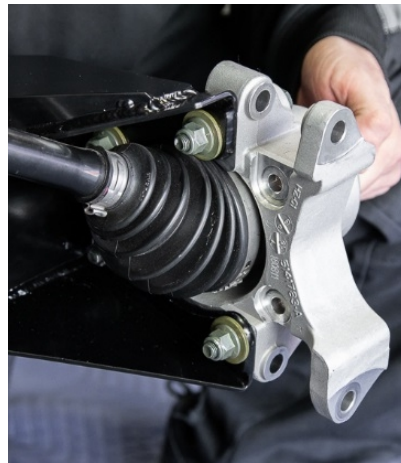
Figure 18B: Axle Installed
