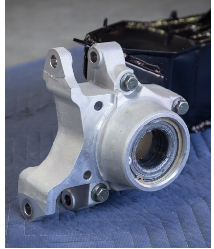
Figure 15C: Bearing Carrier Installed
