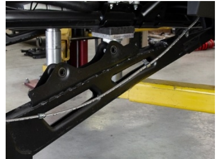
Figure 7C: Brake Line Removed
