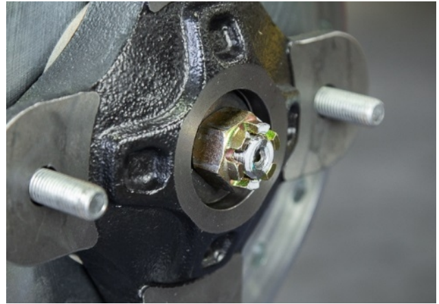
Figure 21B: Hub Nut Installed
