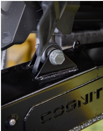
Figure 17A: Sway Bar End Link Installed
