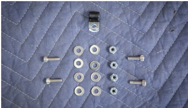
Figure 22: Brake Line Hardware
