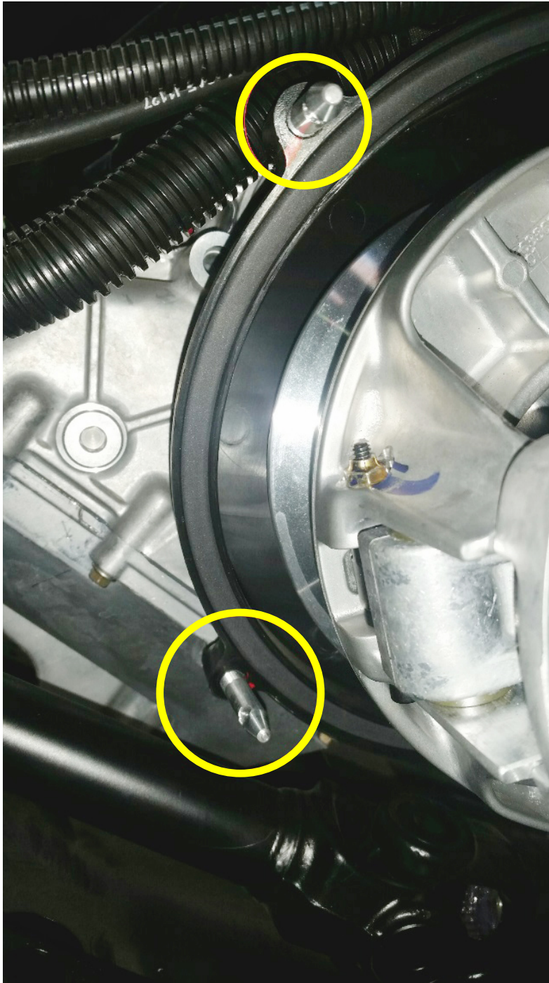
Figure 2: XP1k Clutch Cover Front Two Pin Locations
