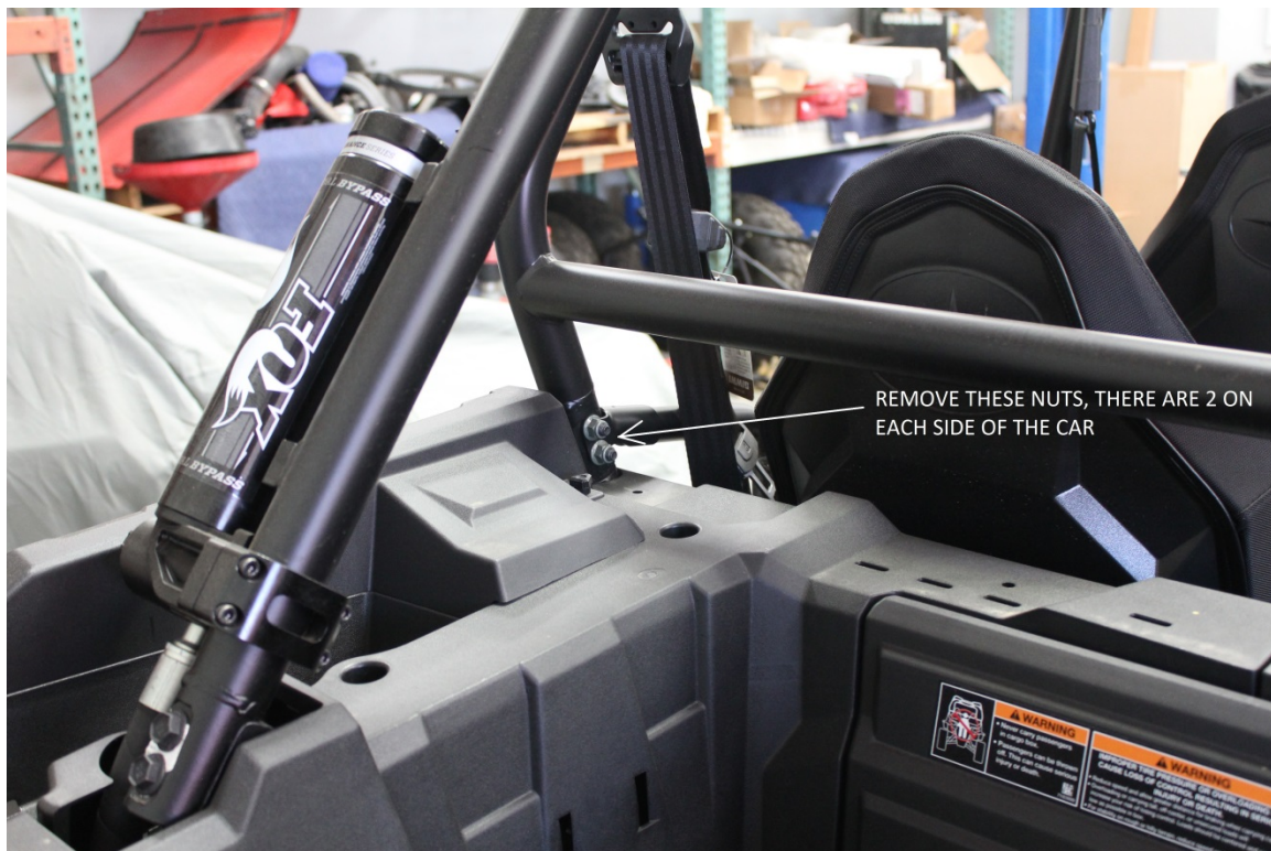
Figure 1: remove nuts, 2 on each side of car
