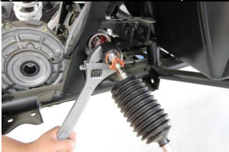
Figure 1: pull dust boot back, remove inner tie rod from rack bar.
