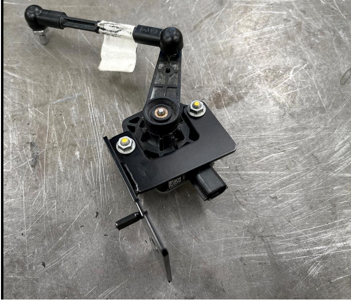
Figure 17: Ride Height Sensor Installed onto Cognito Bracket
