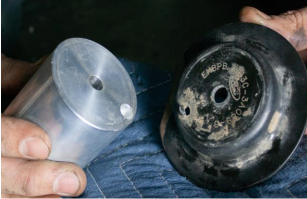
Figure 6: Bump Stop Spacer and OEM Mount
