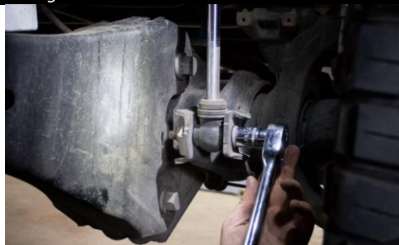
Figure 2: Front Shock Lower Bolt Removal
