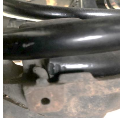
Figure 9: Bottom Spring Pigtail Installation
