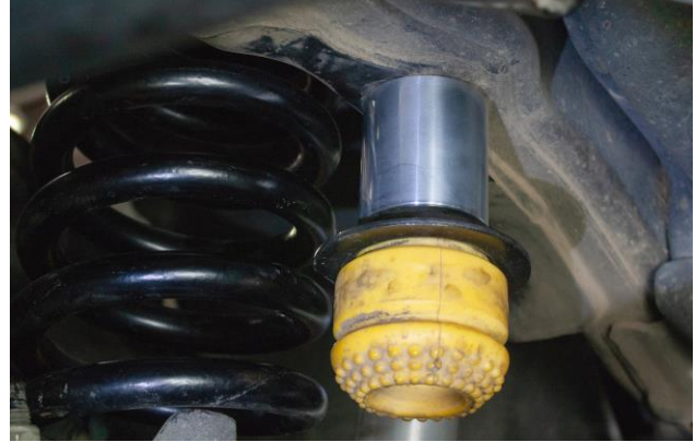
Figure 7: Assembled Bump Stop Installation
