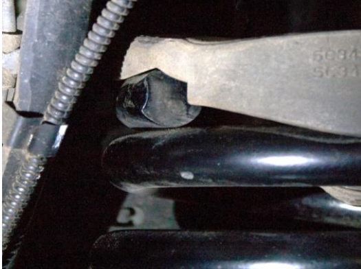
Figure 8: Top Spring Pigtail Installation
