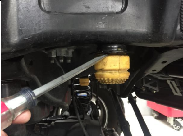
Figure 4: Bump Stop Spacer Removal
