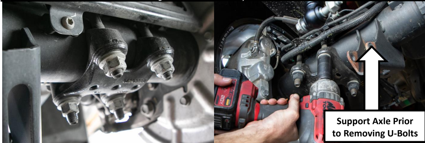
Figure 1: Remove Factory U-bolts.
