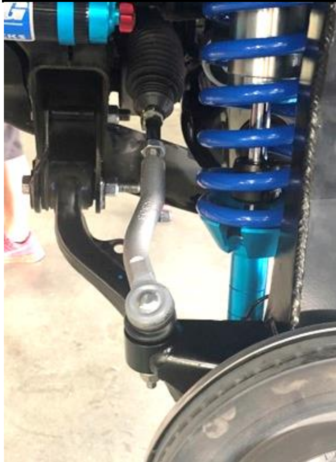
Figure 40: Tie Rod Assembly Attached to Spindle.
