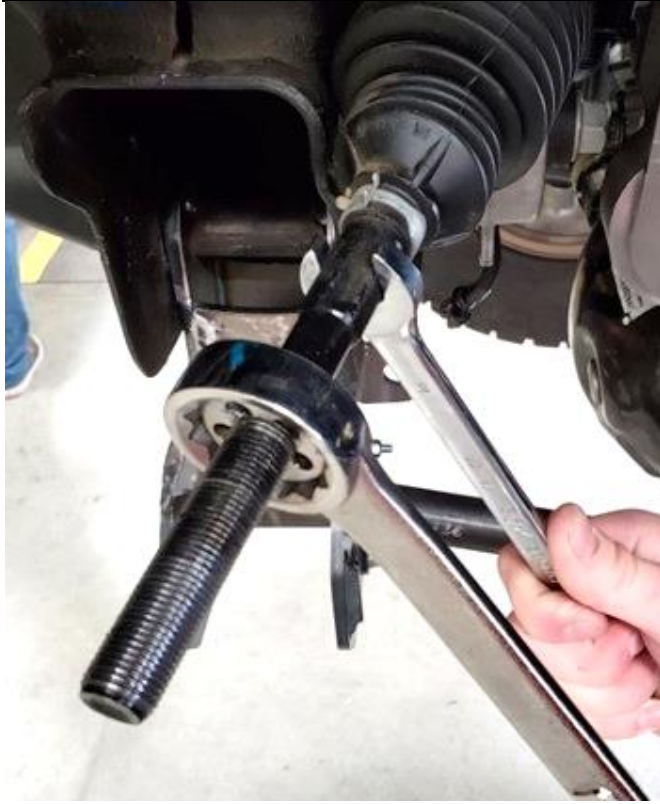
Figure 22: Tread OEM Inner Tie Rod with Die
