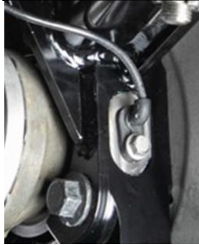
Figure 58: Speed Sensor Installed.
