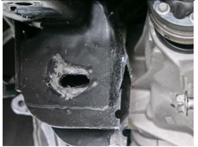
Figure 21: After Cutting Crossmember Mount.
