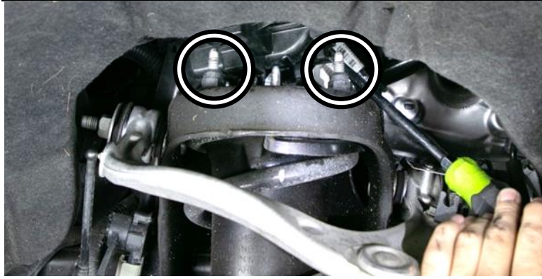
Figure 12: Upper Strut Mounting Nuts. Inboard nut hidden in picture.
