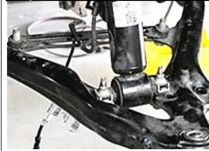
Figure 43: Strut Attached to Lower Control Arm.
