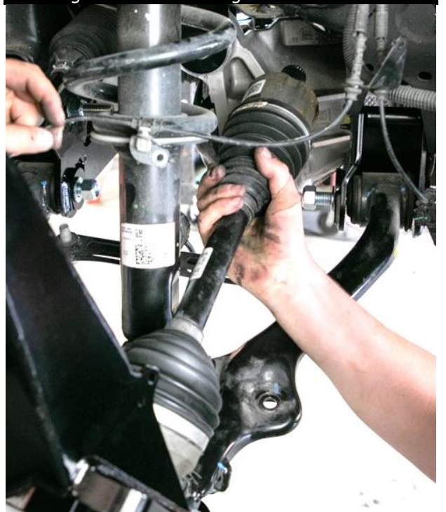
Figure 49: Reinstalling Front Drive Axle.
