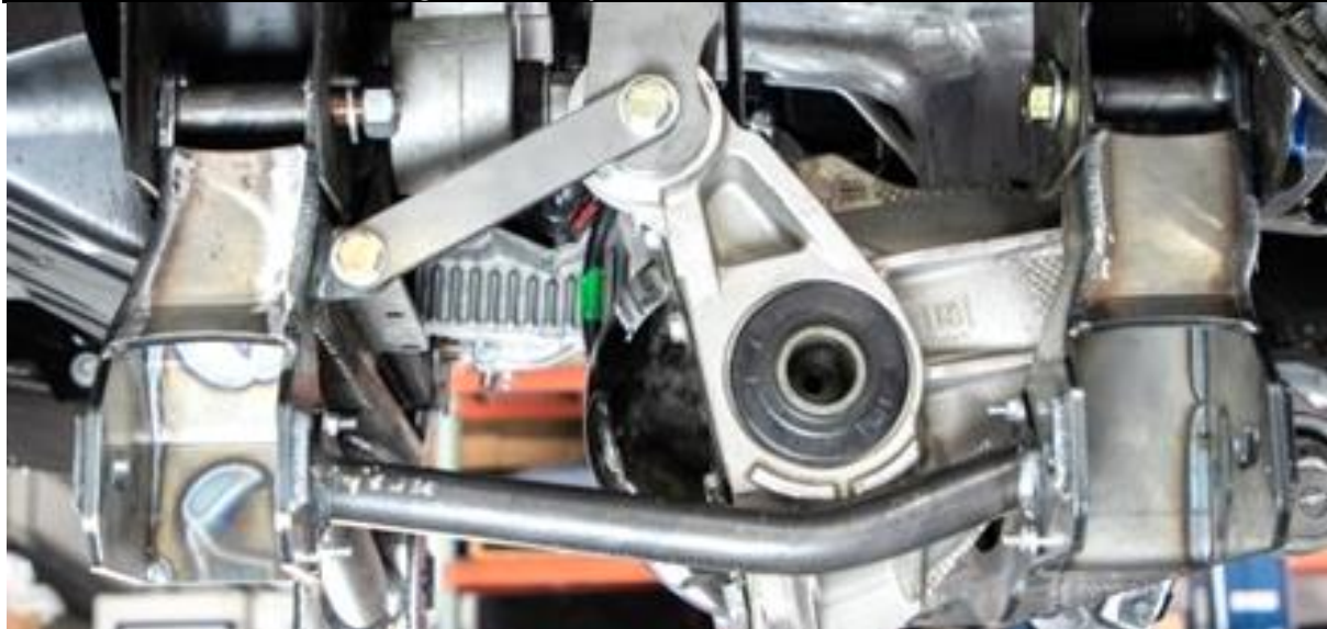
Figure 39: Sub-frame Connector Installed.
