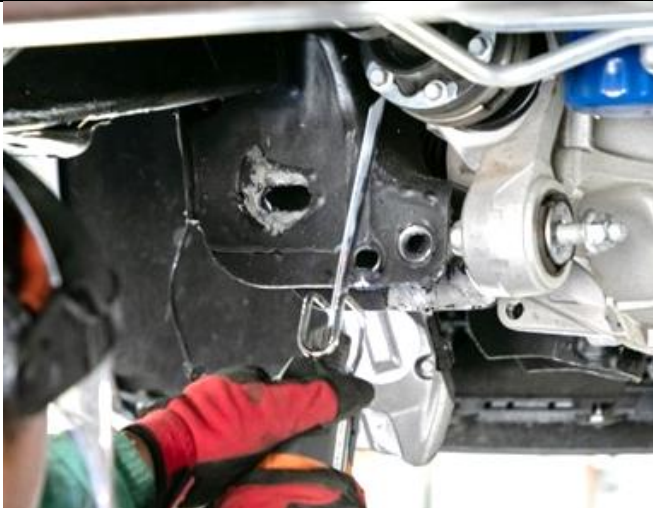
Figure 20: Cut Driver Side Crossmember Mount.
