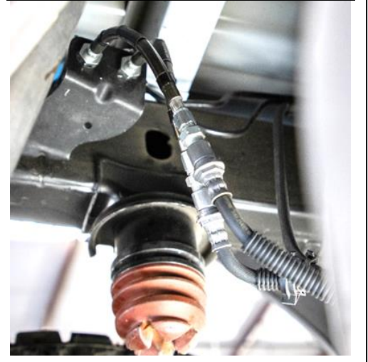
Figure 68: Brake line extension installed.
