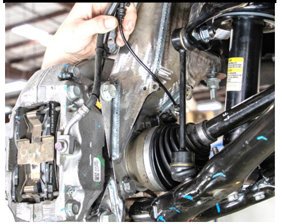
Figure 54: Sway Bar End Link Attached to Lower Control Arm.
