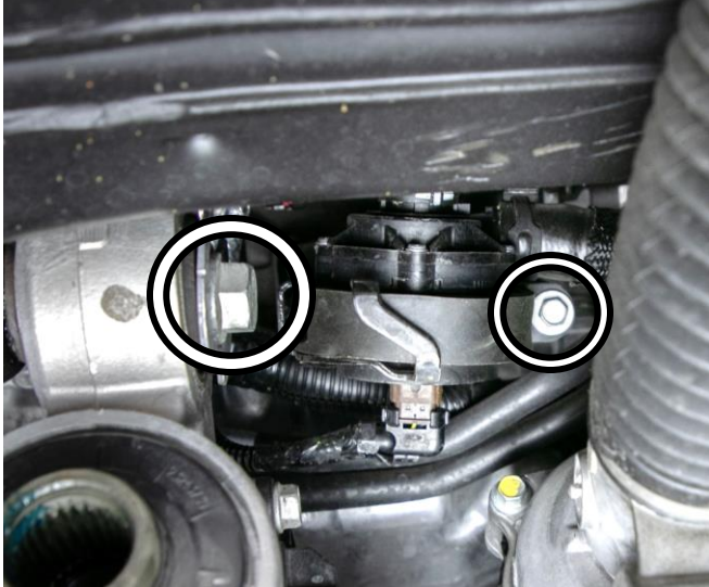
Figure 17: Passenger Side Differential Mount and Actuator. Second actuator bolt hidden in picture.
