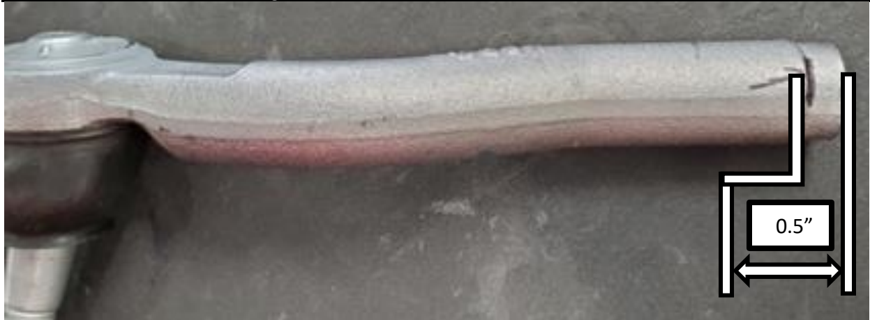
Figure 25: Mark & Cut OEM Outer Tie Rods.
