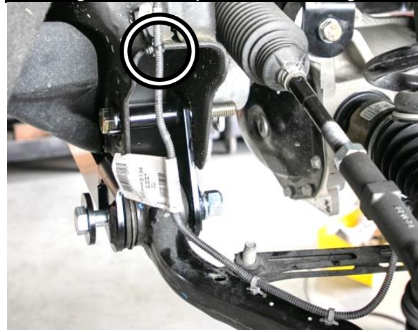
Figure 62: ARC System Wire Routing.
