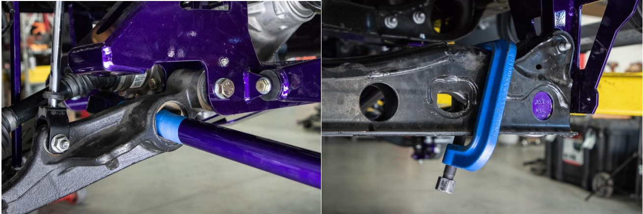
Figure 66: Torsion Bar Installation
