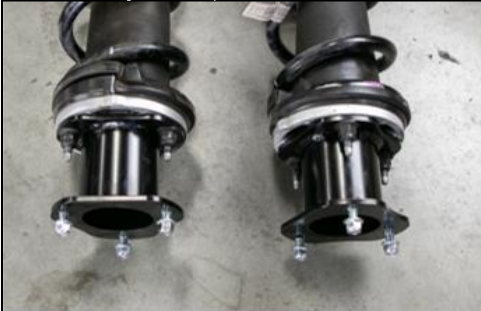
Figure16: Strut spacers installed on struts..
