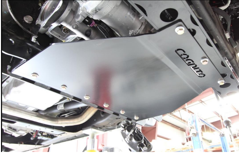
Figure 15: Instal 1923 skid plate.
