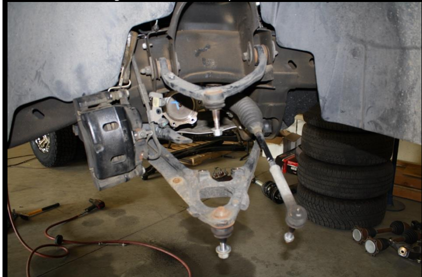
Figure 5: Shock and spindle removed.
