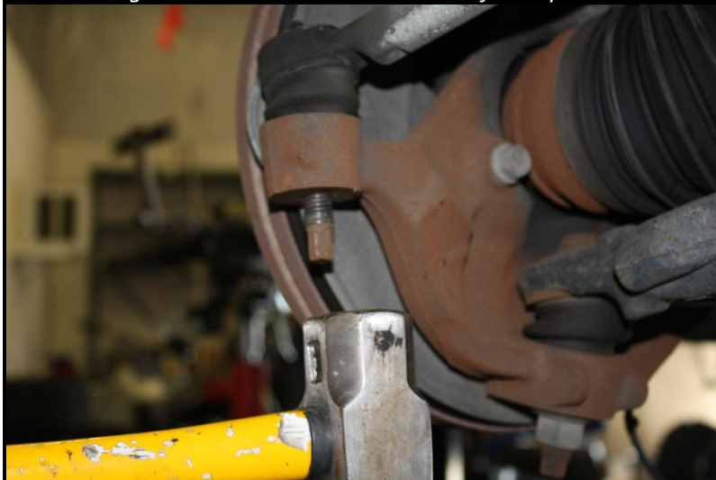
Figure 1: remove outer tie rod end from spindle
