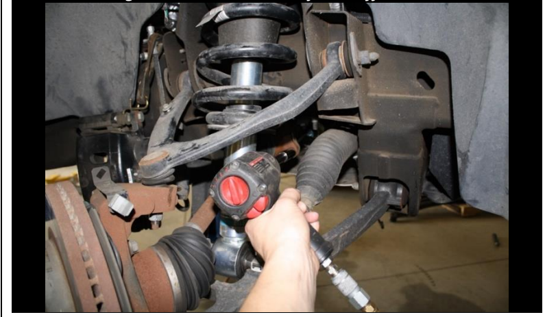
Figure 2: unbolt CV axle from differential
