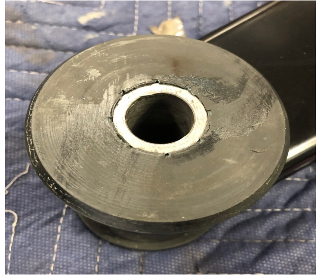
Figure 24: Crush Sleeve Installed
