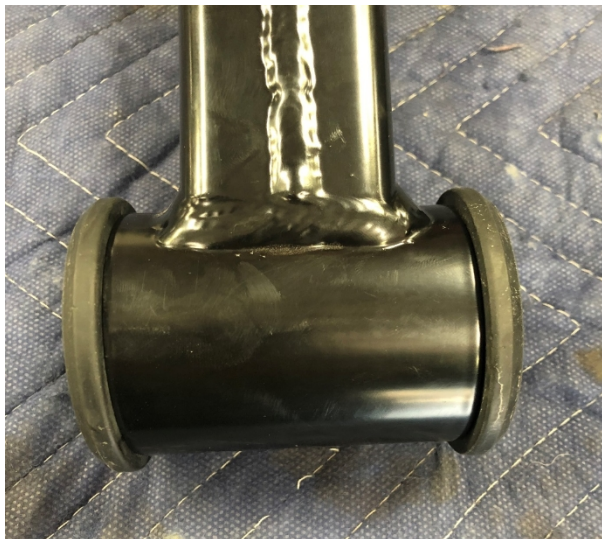
Figure 21: Traction Bar Bushings Installed
