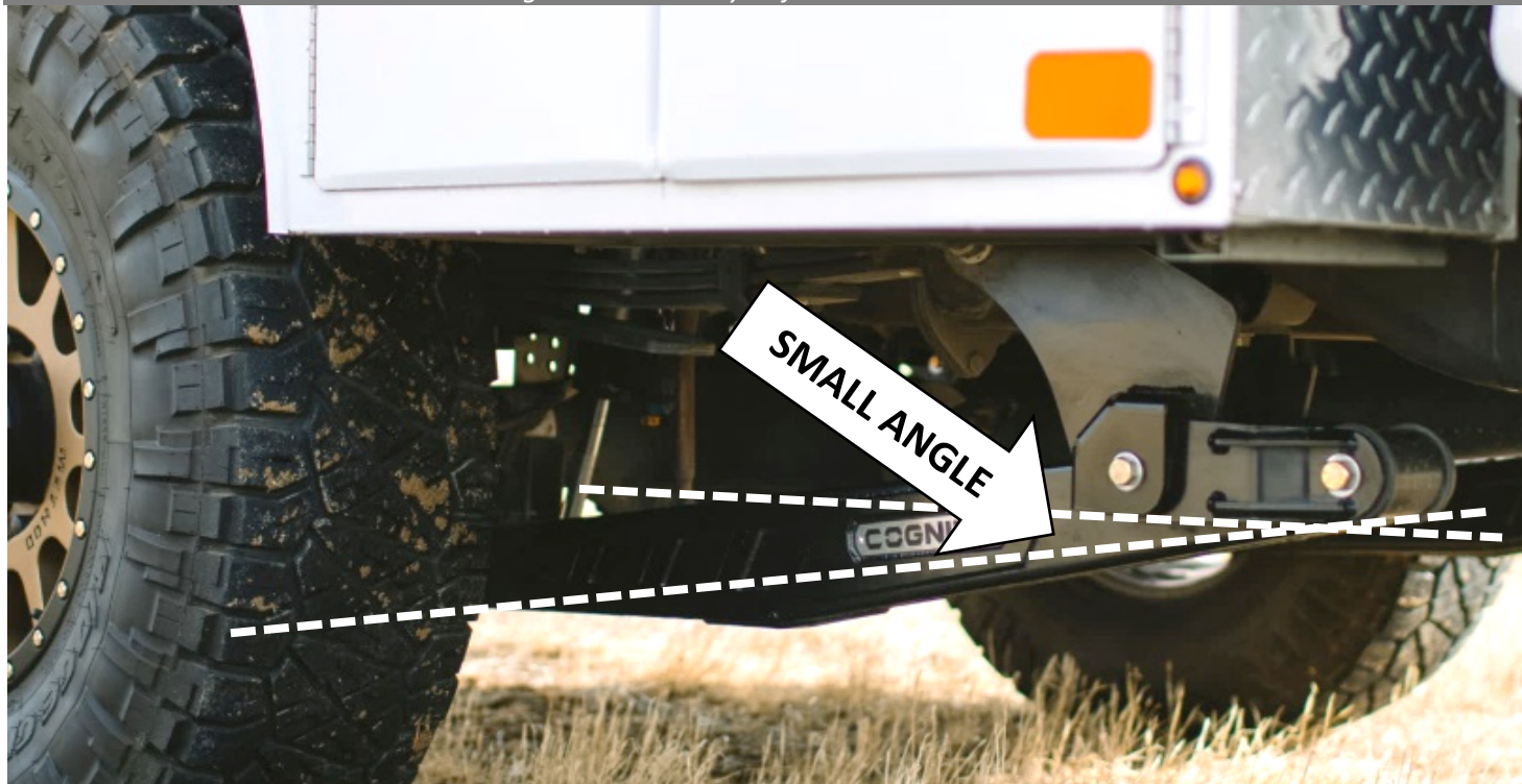
Figure 31: Correctly Adjusted Traction Bars
