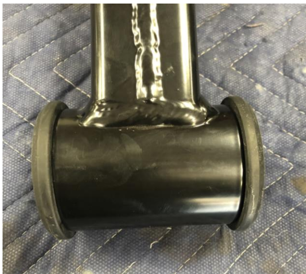
Figure 21: Traction Bar Bushings Installed
