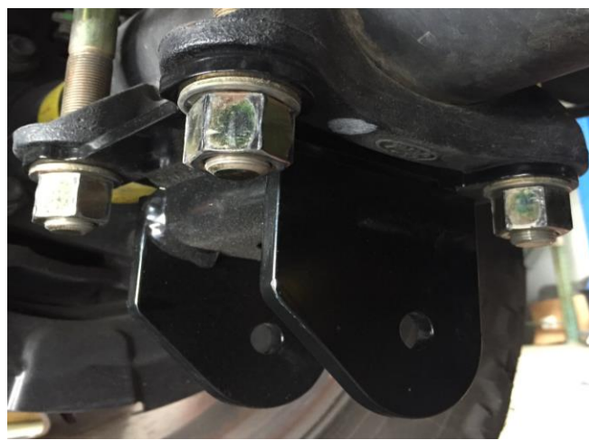
Figure 19: Install Axle Mount Bracket
