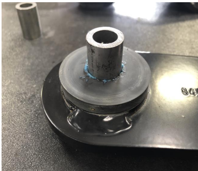
Figure 14: Install Shackle Crush Sleeves
