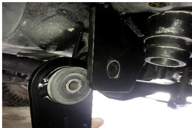
Figure 16: Assemble Shackles to Frame Mount
