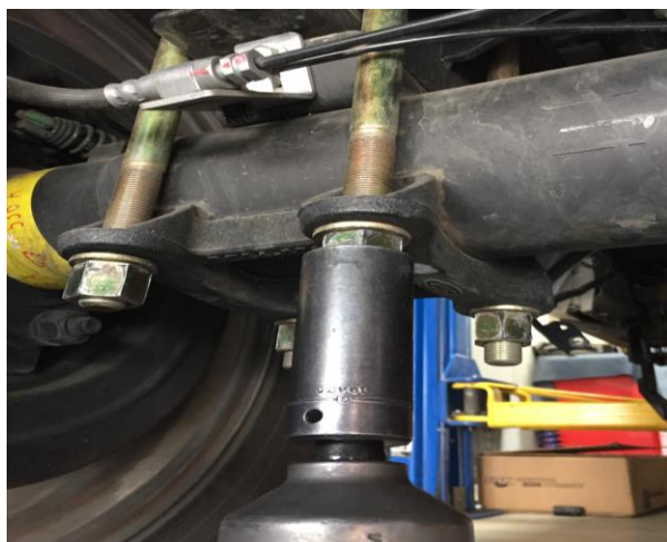
Figure 18: Remove U-Bolt Nuts
