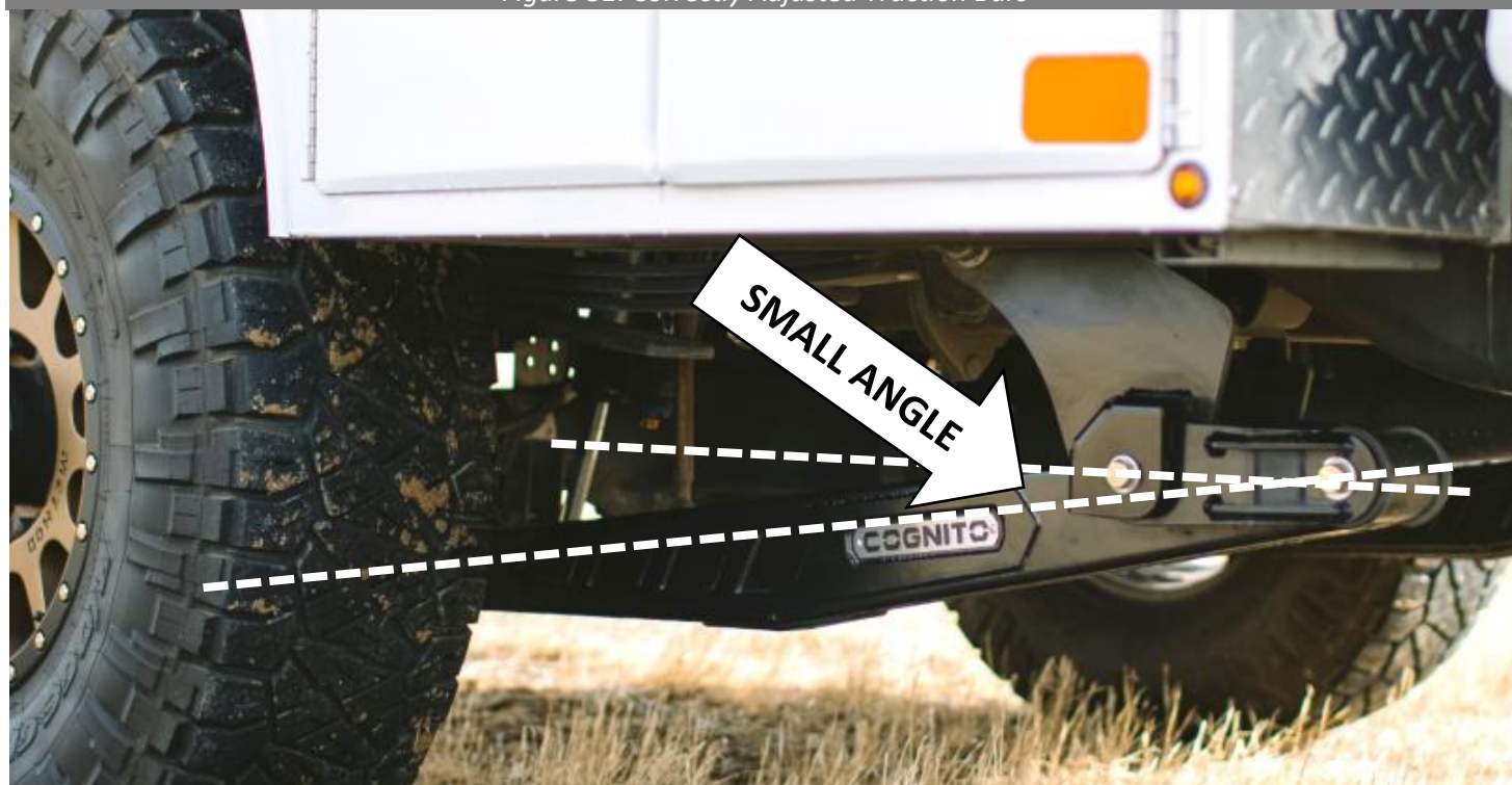
Figure 31: Correctly Adjusted Traction Bars
