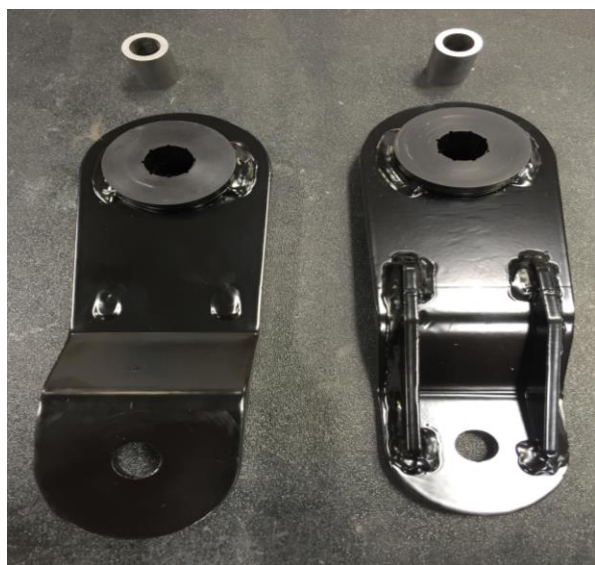
Figure 12: Install Shackle Bushings
