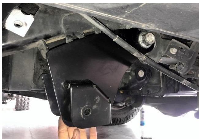
Figure 5: Frame Mount Bracket Alignment
