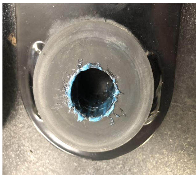
Figure 13: Grease Shackle Bushings
