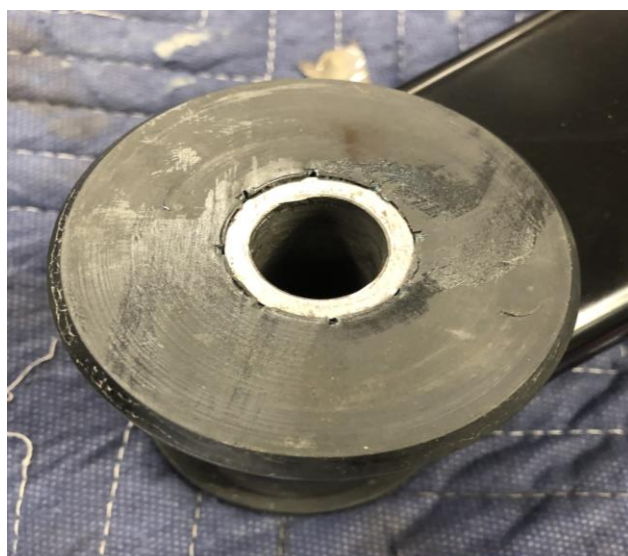
Figure 24: Crush Sleeve Installed
