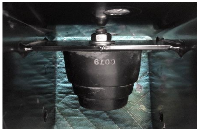
Figure 8: Bump Stop Mounting Nut
