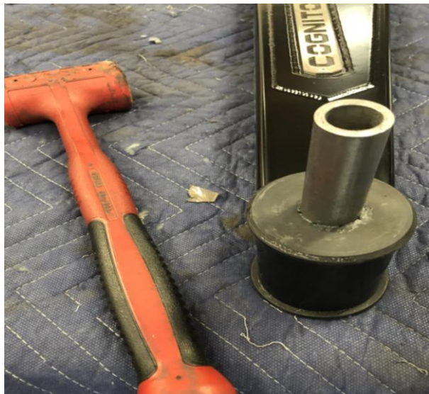
Figure 23: Install Crush Sleeve
