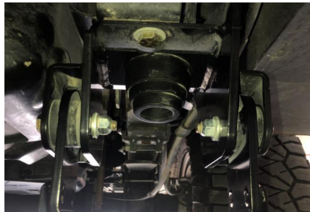
Figure 17: Frame Bracket Assembled
