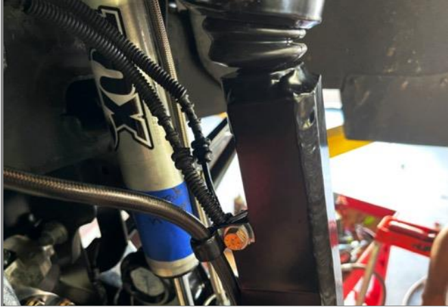
Figure 64: Driver Side Top Spindle Tab & P-clamps
