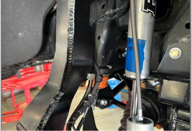
Figure 65: Driver Side Middle Spindle Tab & P-clamps
