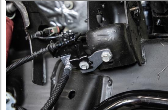
Figure 54: Remove Brake Line Bracket
