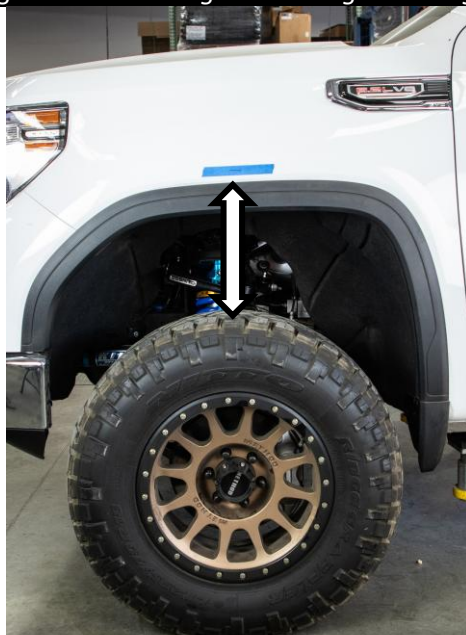
Figure 6: Measuring and Setting Ride Height
