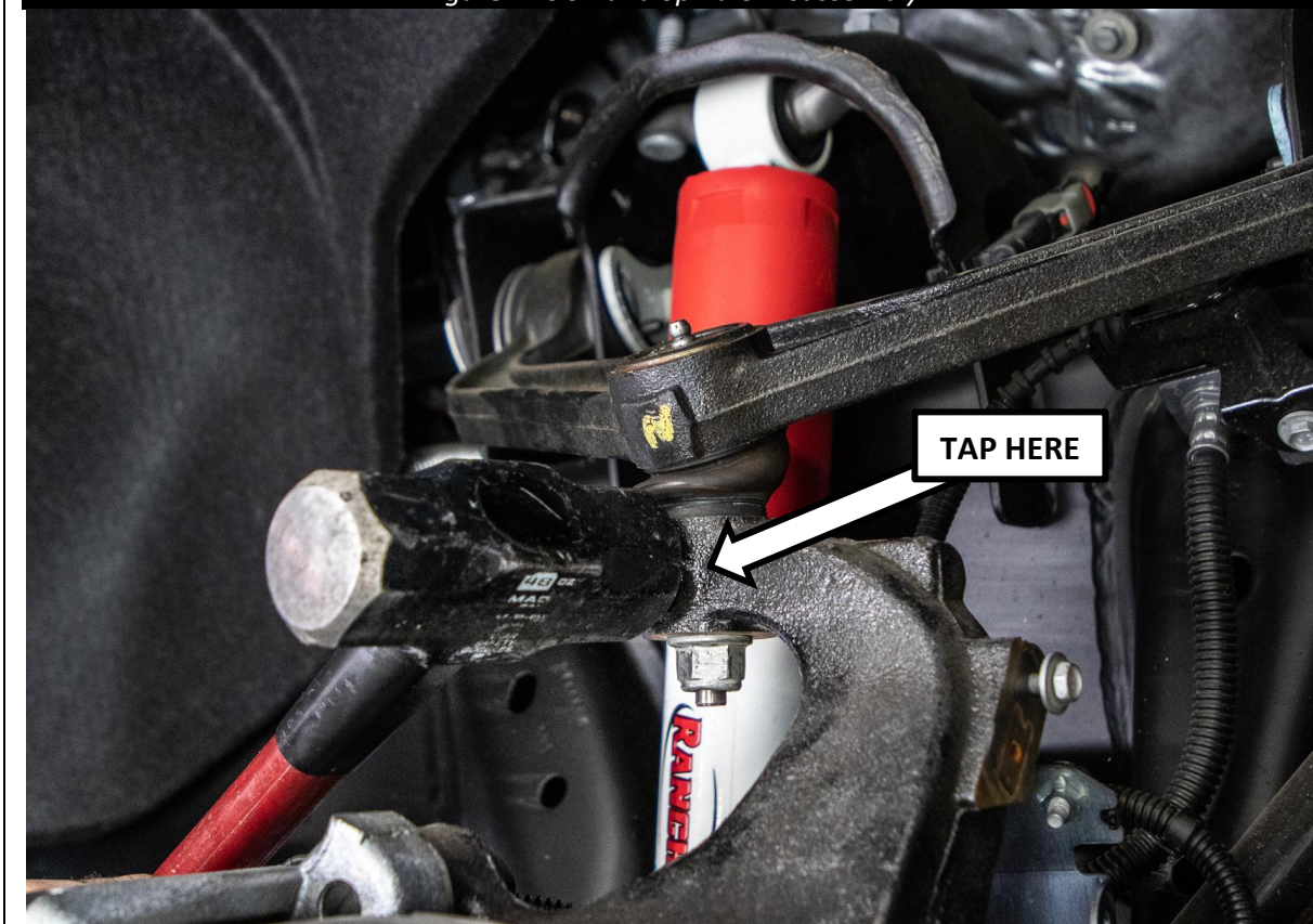
Figure 2: UCA and Spindle Disassembly
