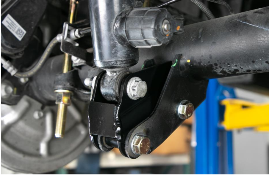
Figure 5b: Bracket Installed
