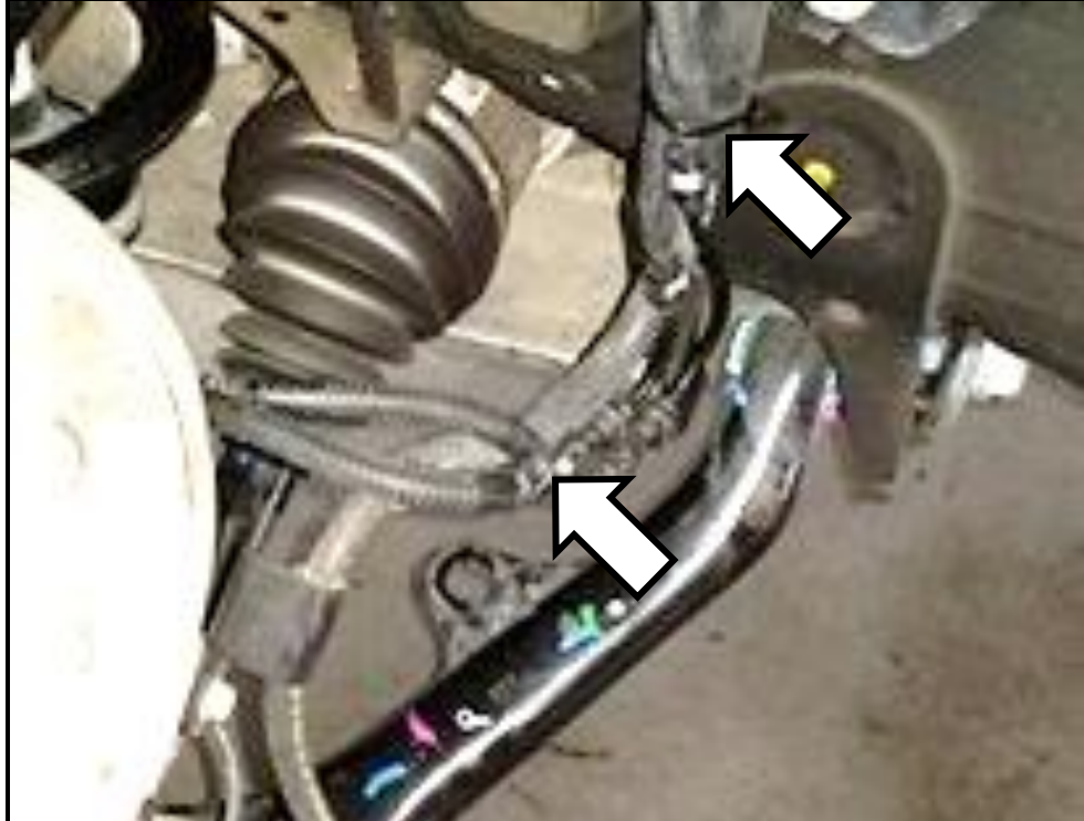
Figure 19: Restrain Wires to Brake Line with Cable Ties
