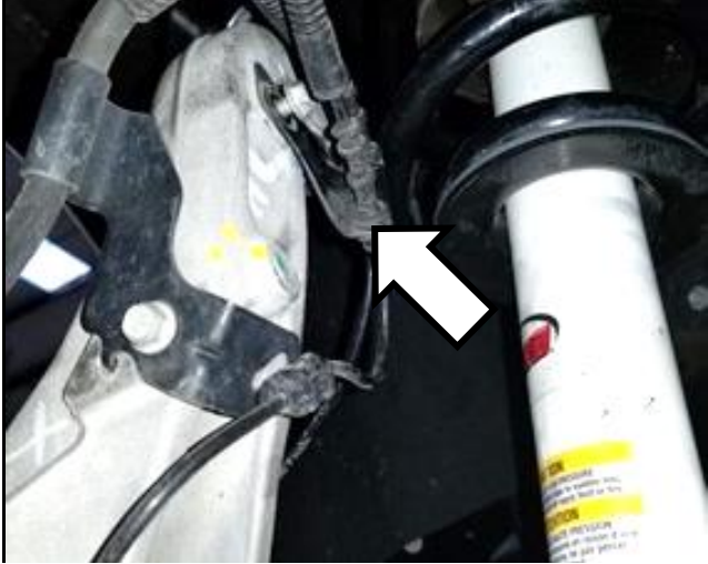
Figure 17: Remove Wire Routing Bracket
