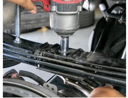
Figure 22: Removing Tapered Shim.
