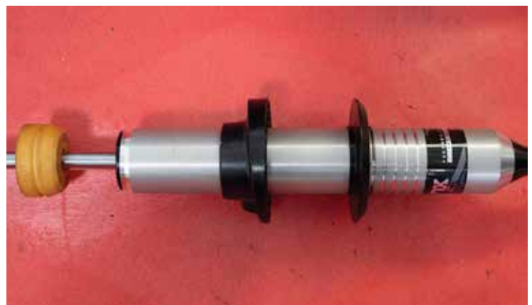
Fig. 17: Install the OEM rubber bumper on the shaft.
