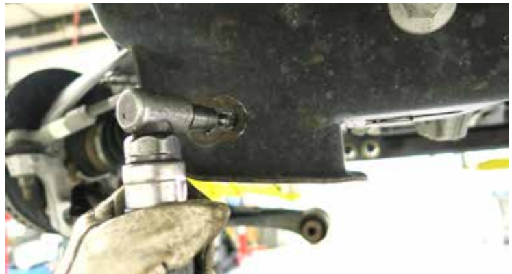
Fig. 11: Slot with a die grinder
