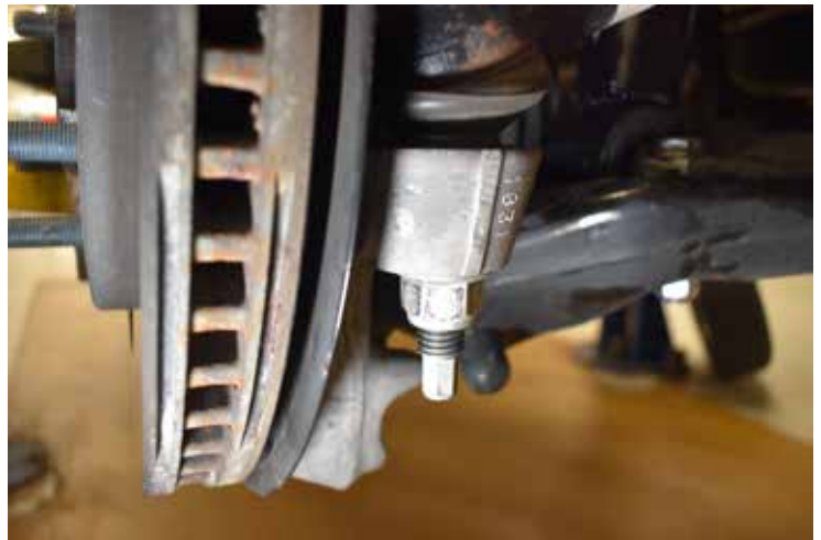
Fig. 23: Attach tie rod to knuckle
