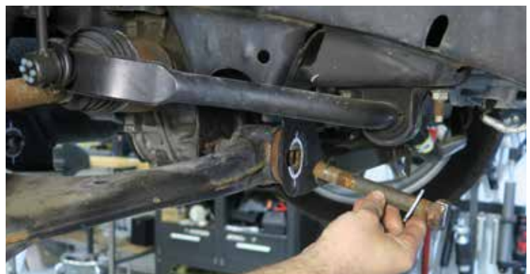
Fig. 6: Lower control arm rear bolt removal.
