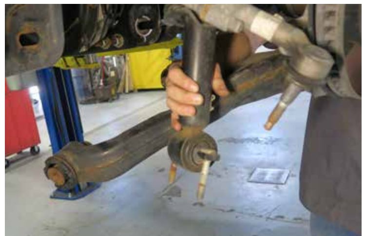
Fig. 9: Remove strut from vehicle.
