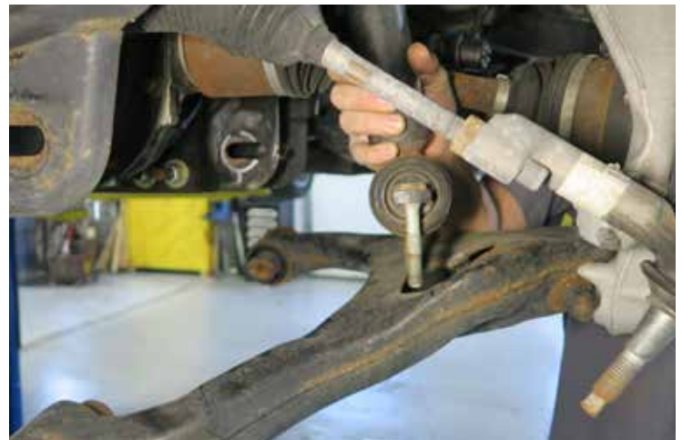
Fig. 8: Remove lower strut from lower control arm.
