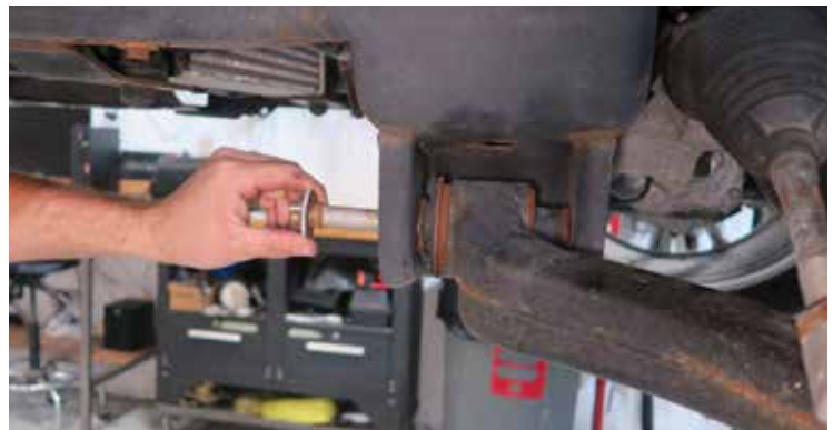
Fig. 5: Lower control arm front bolt removal.
