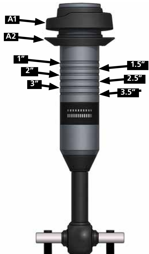
Fig. 16: Lowering heights are approximate due to differences in exact truck configuration.
