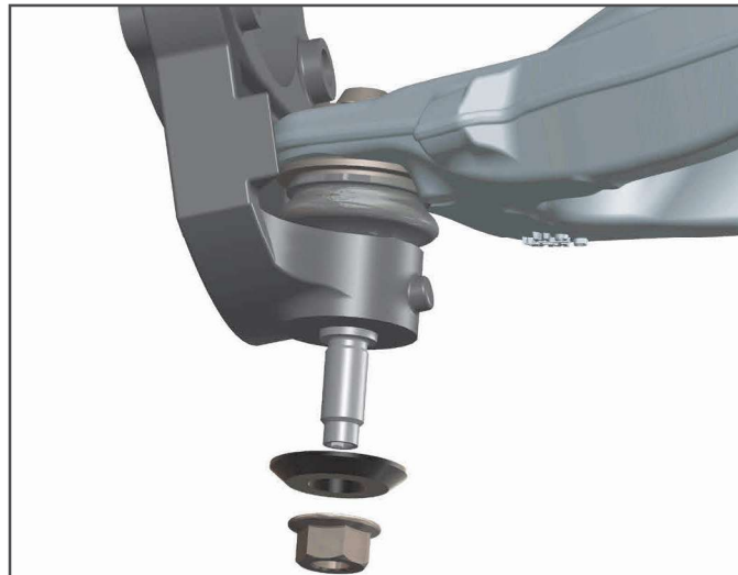
FIGURE 37 - STOCK ALUMINUM/STAMPED STEEL CONTROL ARMS ONLY
