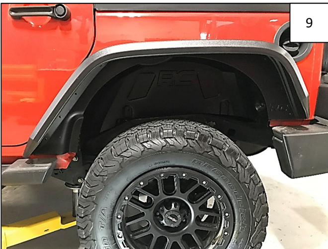
Completed Wheel Well Liner and Flare 99037 installation. Repeat for other side.
