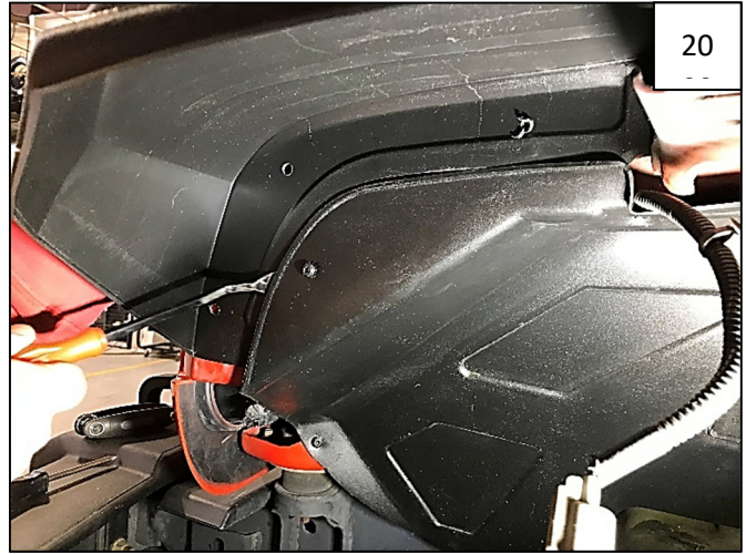
Install flares to instruction for 99037. The front of the flare will tuck slightly under the Wheel Well Liner (ahead of inner fender bracket) as shown. Use a pry tool to help seat the part.
