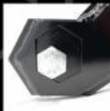
Highest caster setting +6° over stock (5"-6" Lift with no drop bracket)
