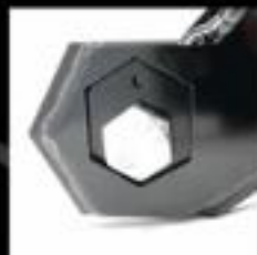
Midway caster setting +4° over stock (3"-4" Lift with no drop bracket)
