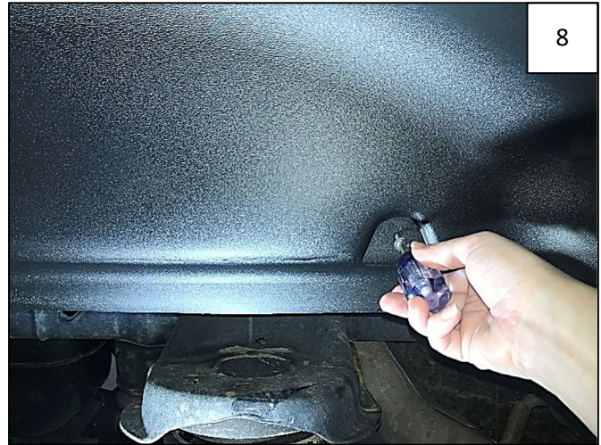
Start a supplied Truss Head Screw through each hole in back of wheel well liner and into clips installed in Steps 3-4. Tighten both screws.
