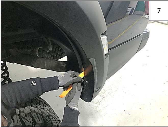
Use a Pry Tool to assist in seating the edge of the Wheel Well Liner along the entire edge.
