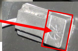
Magnet needs to line up with this emboss
