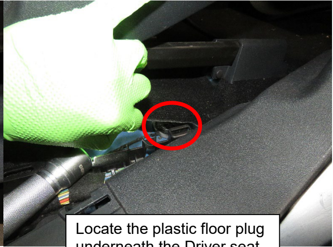
Move the plastic trim to the side
