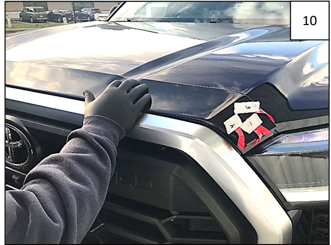
Lower part onto hood, maintaining centered position. Once the tape begins to contact the hood, adhesion is immediate.
