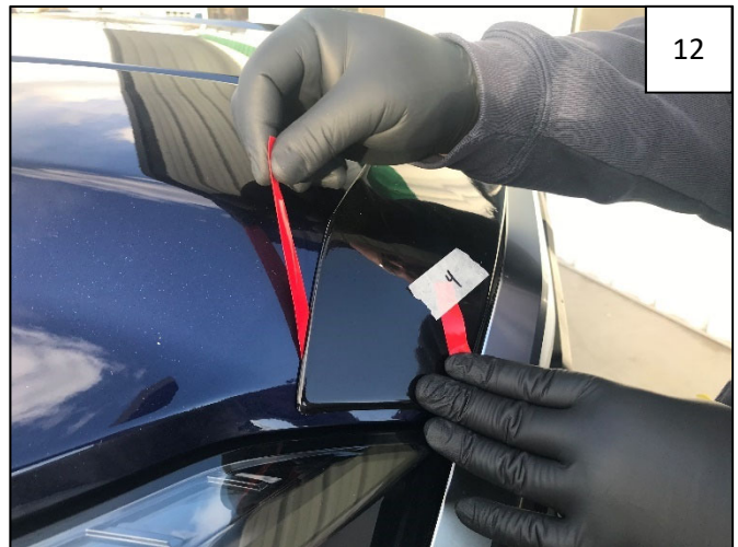
Pull tape leader "3" from each end. Carefully pull each tape leader at a 45-degree angle away from part to release from the tape, pressing against part as you go.
