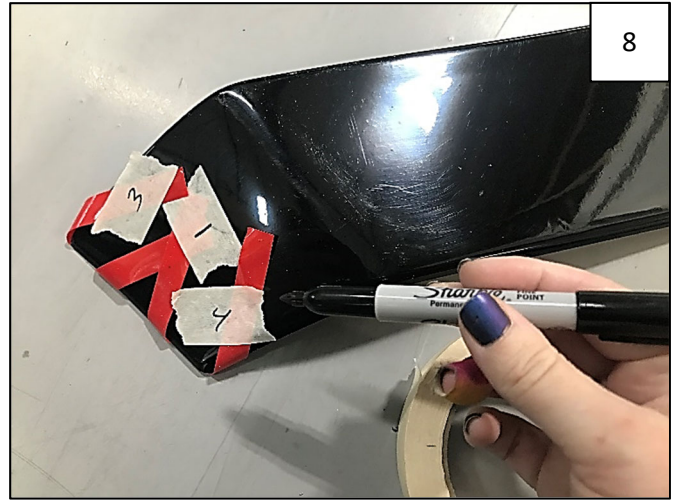
Fold the leader from the other long piece of tape over and secure with masking tape; mark this leader "4".
