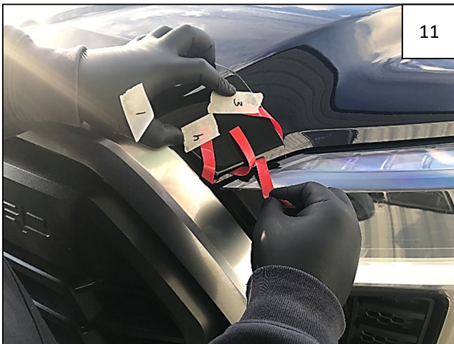
Pull red tape leaders numbered "1" and "2", discarding masking tape, then press each end of part into place.
