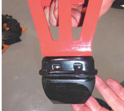
19. Install the factory bump stop cups onto the new bump stop drop brackets using the provided 3/8" allen bolts.
