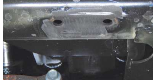
17. Use the provided tap on the existing holes that were located under the factory bump stop mount on the frame. (pic 16)
