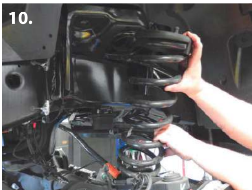
11. Slowly lower the front axle until the front coil spring tension is released.
