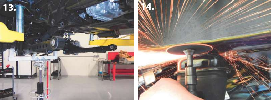
14. Remove the factory radius arms. Use a 27mm socket on the upper arm to axle bolts and a 24mm socket on the lower arm to axle bolts. Use a 27mm socket on the arm to frame bolts. (pic 13)
