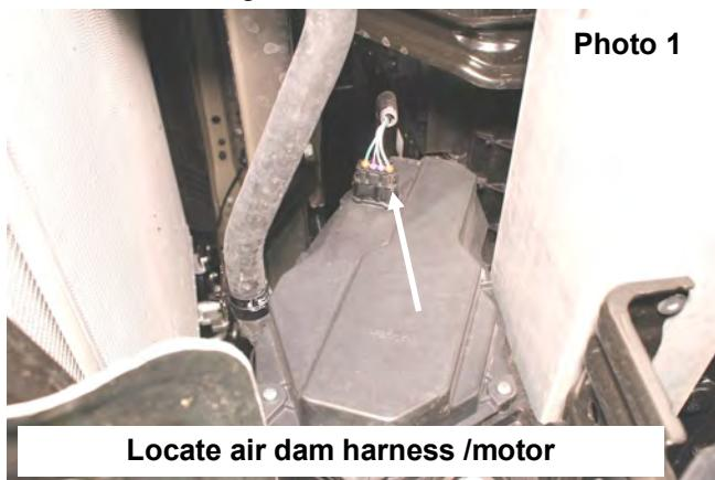
Locate air dam harness /motor
