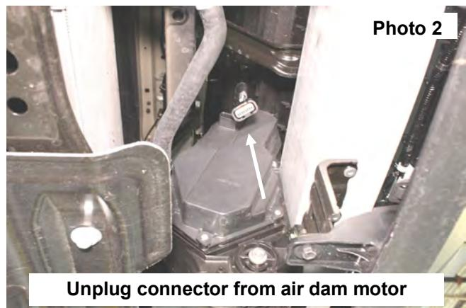
Unplug connector from air dam motor
