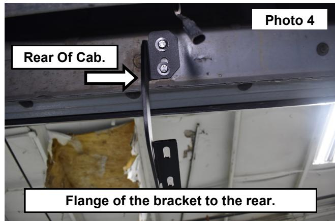
5. Install the (2) Rear bracket to the cab. Secure the bracket to the cab mounts using (2) of the supplied Hex head bolts, (2) Flat washers and (2) Lock washers. **See Photo 5.**
