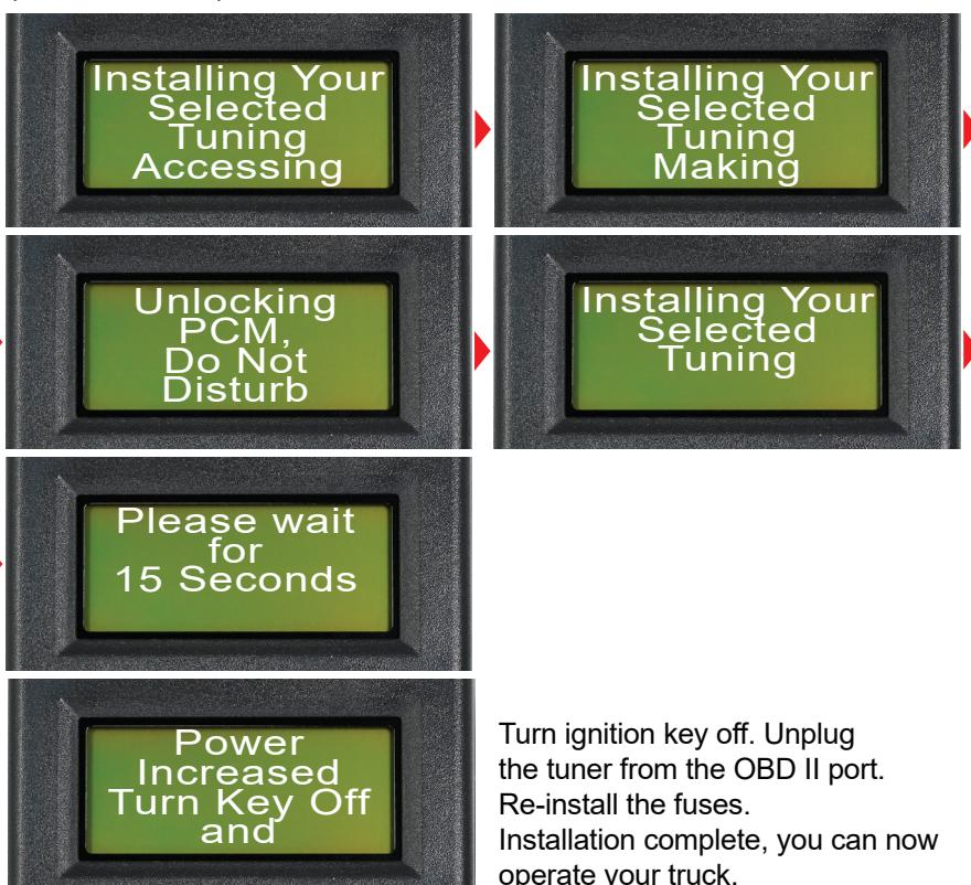
Turn ignition key off. Unplug the tuner from the OBD II port. Re-install the fuses. Installation complete, you can now operate your truck.
