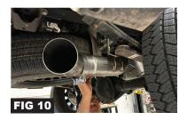
Step 9. Install 4" Exhaust Clamps (G) onto the 5" Exhaust Tip (F). See (FIG 11 & FIG 12).
