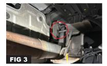
Step 3. Remove the stock exhaust from the exhaust insulators. See (FIG 3 & 4).
