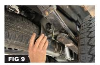
Step 8. Install the 4" 90 Deg Pipe **(E)**with the 4" Exhaust Clamps **(G)**.
