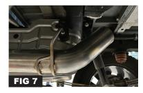
Step 7. Install the 4" Over-Axle Pipe (D) with the 4" Exhaust Clamps (G). Secure hanger on the exhaust insulators. See (FIG 8 & FIG 9).
